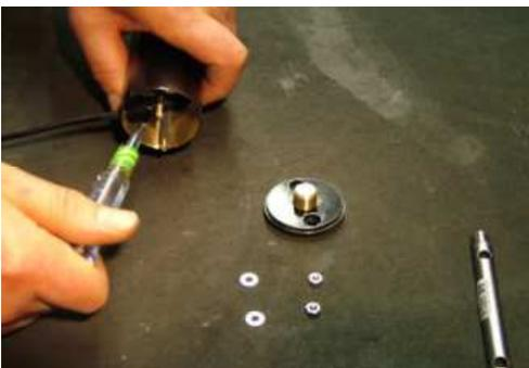
4. Loosen the strain relief device.
