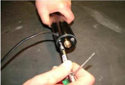
2. Use the socket spanner to loosen the nuts.
