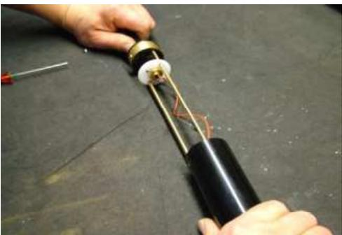
6. Hold the arm and remove the shaft.
